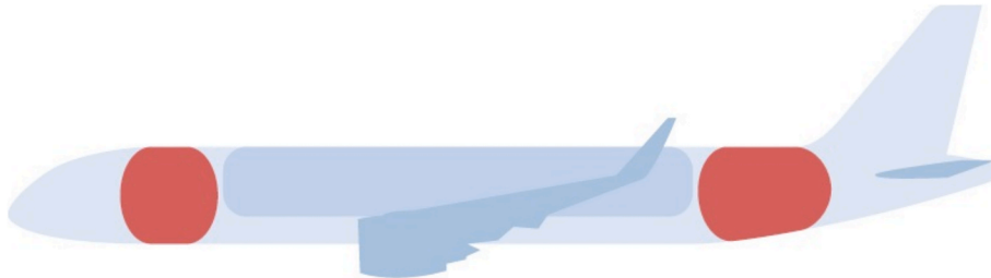
Fig. 2. The structure of a non-integral tank carries hydrogen fuel used in the present study. The design of the hydrogen storage tank includes a hatch to ensure access to all regions of the aircraft.
